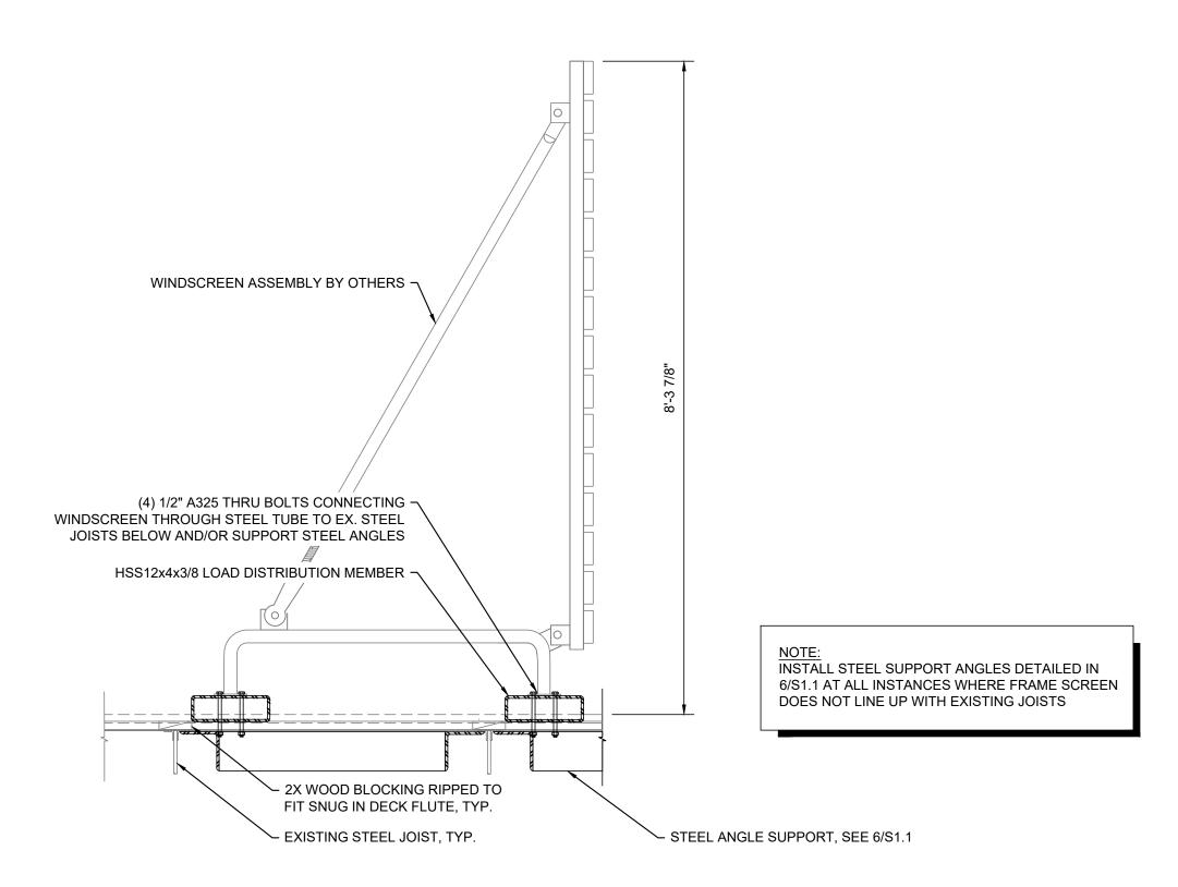
FRAME SCREEN SECTION (PARALLEL TO JOISTS) ARCH REF: 6/A-5.2
